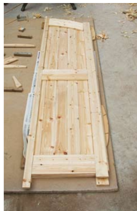
▲ Pic.3 The three layer lamination can be seen here, before the horns are trimmed
