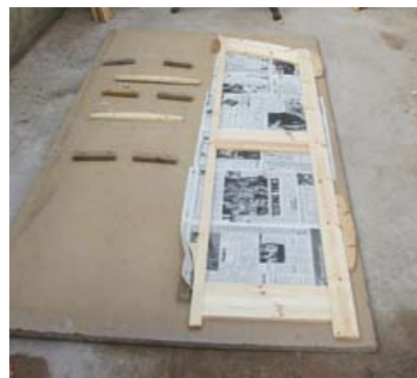
▲ Pic.2 A sheet of old chipboard serves to keep everything aligned
